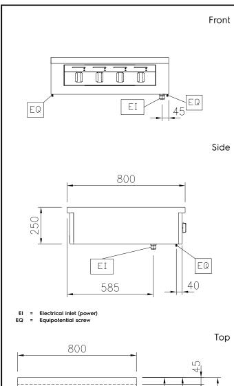
**Electric** Supply voltage: 400 V/3N ph/50/60 Hz **Total Watts:** 20 kW
